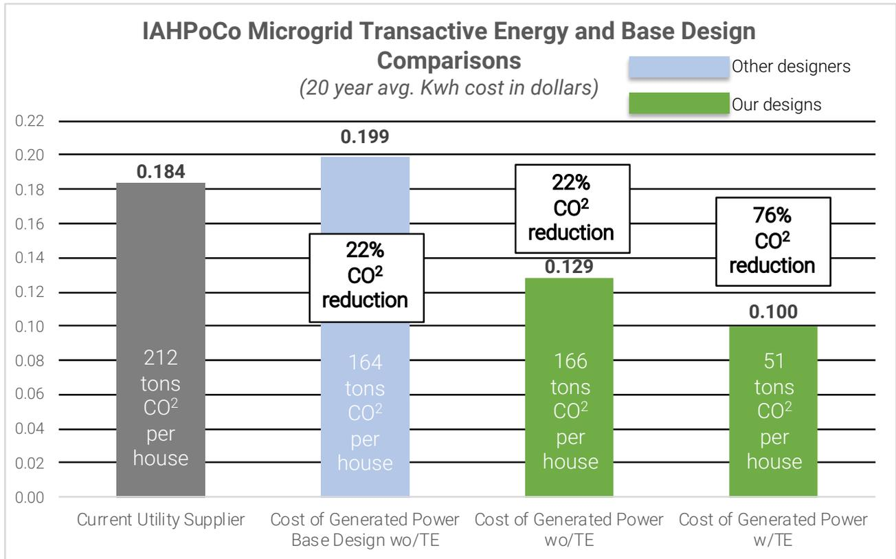
When Introspective System's transactive energy controls are added to the microgrid, further increases in energy efficiency, renewable energy utilization, and peak shaving can be achieved. In certain applications, like on IaH, significant additional carbon dioxide reductions can be achieved by offsetting fossil fuel space-heating with renewable power that would otherwise be curtailed in typical microgrids with very high renewable penetration (microgrids aiming for above 70% renewable generation).
